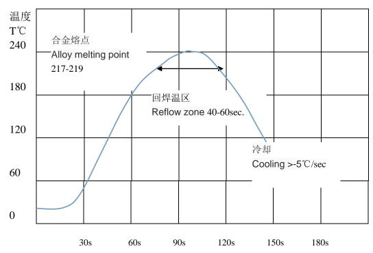
Reflow oven: Heat cure according to the reflow curve as shown below.
