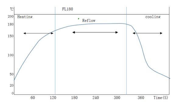
Heating: $25^{\sim}150^{\circ}\text{C}$ ,  $2-3^{\circ}\text{C/sec}$ Reflow:>150°C, 180-240sec
